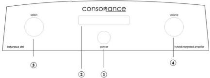
The amplifier is switched on with the button ① ②Display. By pushing the same button one more time the power is switched off.
